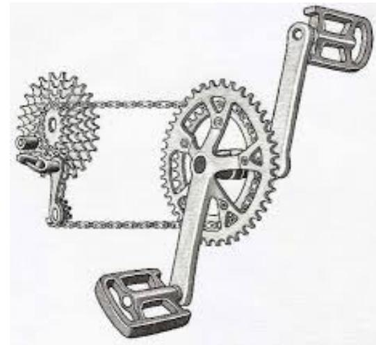
Sometimes gears are connected by a chain.
